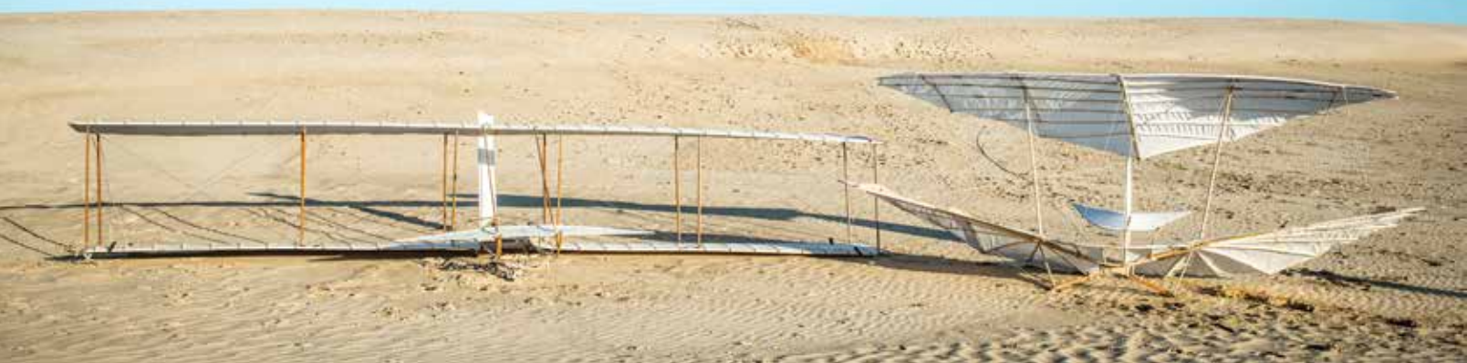
ABOVE Andrew Beem flying Otto Lilienthal's "Großer Doppeldecker" next to a modern offspring. Photo by Markus Raffel for DLR. BELOW From the very first repeated human flights with birdlike wings to a controlled flying machine ready for engine integration: Otto's glider (right) and what the brothers made out of it in just 7 years (left). Photo by Arno Trümper for DLR.
